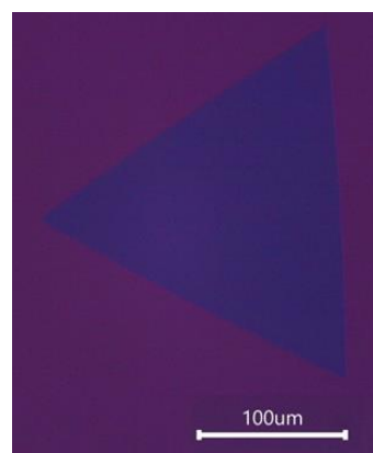
Figure 5. Optical Microscopy image of the as-grown WS_2 flake on SiO_2/Si substrate using solution precursor under optimal achieved condition.
