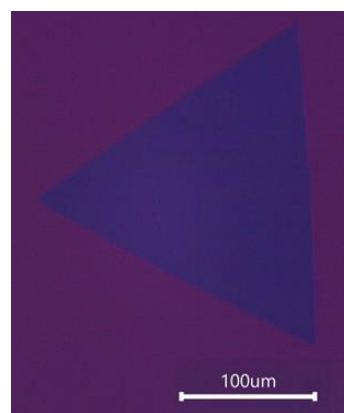
Figure 5. Optical Microscopy image of the as-grown \text{WS}_2 flake on \text{SiO}_2/\text{Si} substrate using solution precursor under optimal achieved condition.
