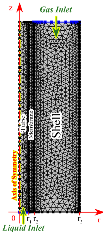
Figure 3. The meshed geometry that is used in the HFMC system simulation in COMSOL Multiphysics software.
