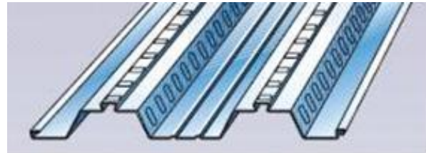
(b) Trapezoidal steel decking profile KF70
