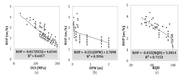
Figure 4. The correlation between penetration rate and rock mass parameters
