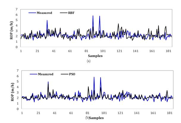
Figure 9. Results of models; Comparison of measured and predicted values of ROP (a) RBF, (b) PSO
